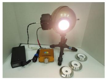
UIS-LS System provides uniform and constant spectral output. Accessories such as power control module and Iris set can be chosen to provide stepped output.
