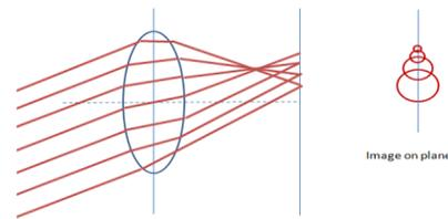
Figure 2: Diagram of coma caused by a lens. Graphic on the right shows the characteristic “comet tail” that is seen in coma aberrations.
