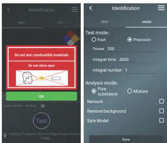
Step 4: Press the test button to collect sample data. While testing, do not move the sample until the result is displayed.
