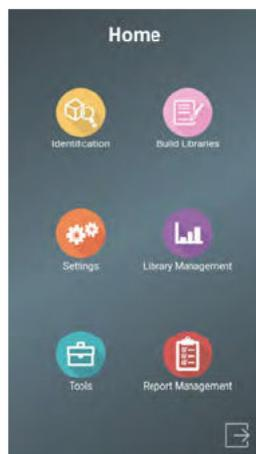
Click the 'Identification' button on the homepage to enter the Identification interface. For a liquid sample, use the liquid sample holder. Then click the 'Test' button. Do not remove the sample during the test. The screen display will switch from 'Testing' to 'Comparing'. When you view this page for the first time you will see a safety prompt to confirm the laser is not aimed at eyes or on skin. Then click the 'OK' button.
