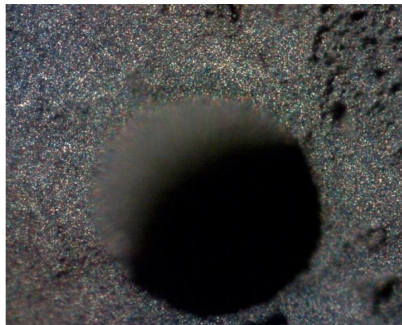
Unfortunate Graphene sample with laser hole
