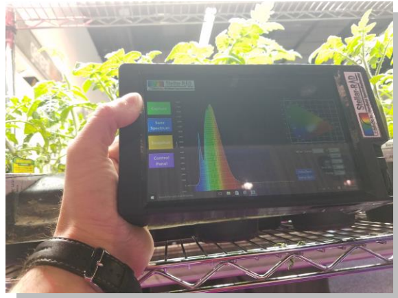
The StellarRAD Handheld SpectroRadiometer measures the spectral output of different grow lights
