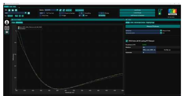
Fig 3: Silicon Nitride (SiNx) Anti-Reflection Coating
