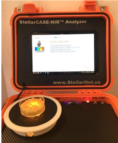
Figure 2. StellarCASE-NIR with corn sample.
