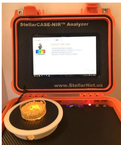
Figure 2. StellarCASE-NIR with corn sample.
