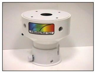
RFX-3D Reflectance fixtures have integrated halogen light source to make color measurement easy by placing samples on top
