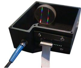
High performance spectrocolorimeter has internal concave grating spectrograph optics with no mirrors or adjustments
