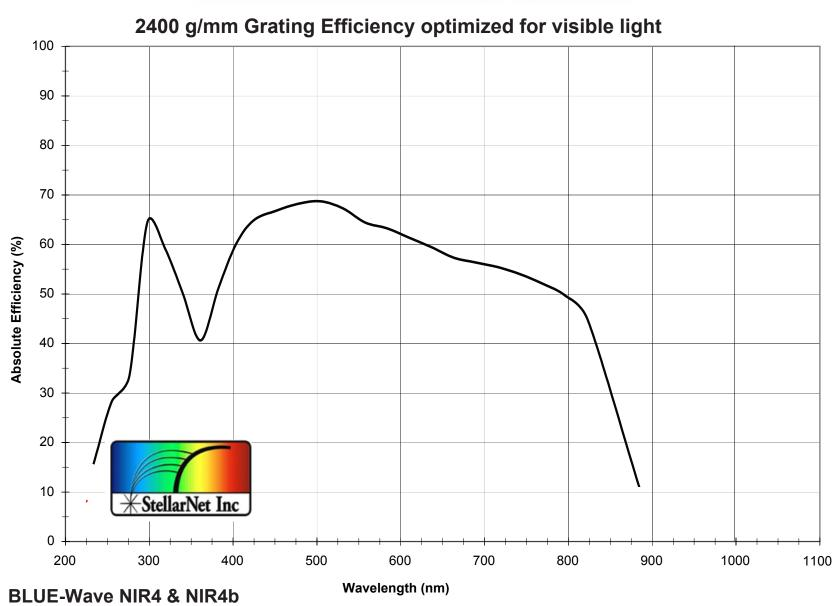
\*Note - Doesn't include contributions from detector or other optical elements Should also review system sensitivity curves as well
