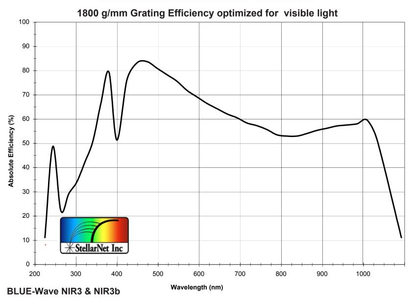
\*Note - Doesn't include contributions from detector or other optical elements Should also review system sensitivity curves as well
