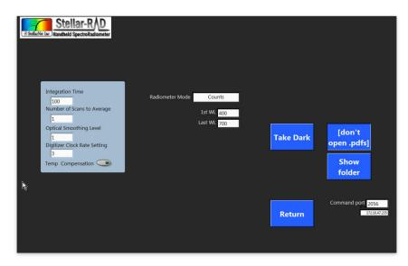
To adjust a parameter: click in its field, type in or select the desired value, then press the Return button. To take a dark spectrum, click its button on either the main operating panel or the Control Panel, and follow the on-screen instructions.
