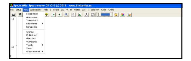
Scope mode: Displays uncompensated/relative spectral data
