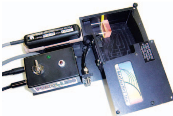
Figure 2: PORTA-LIBS 2000 system photo: sampling chamber, laser, and timing circuit
